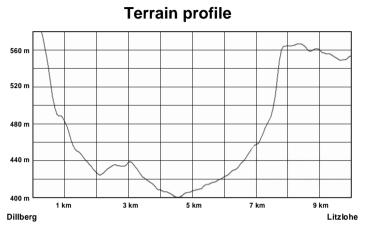
⇒ Representation of the terrain height with only ONE value for a transmitter results in great differences
