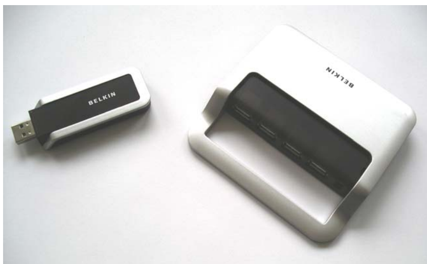
Abbildung 6.5: Cable-Free USB Hub der Fa. Belkin International, Inc.; links: USB-Dongle, rechts: Hub
