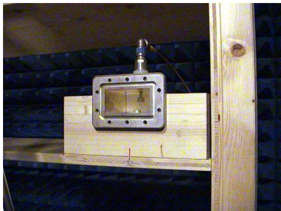
(a) UMTS antenna placed for measurements without animals. Position “front”
